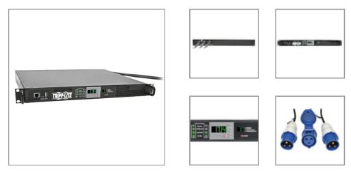
High-capacity 7.7kW PDU with ATS provides remote power monitoring and enables redundant power for non-redundant hardware. Digital display and Ethernet interface allow site power status monitoring for primary and secondary inputs, plus load level monitoring to prevent overload conditions.
